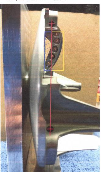
This cut-away of a Polaris clutch with Indy Specialty Clutch Master weights is to help you understand the dynamics of our adjustable weights.
